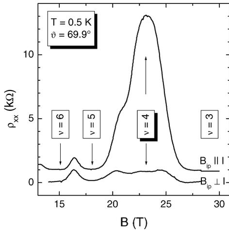
Fig. 3. Resistivity  $\rho_{xx}$  in the centre of the first-order coincidence around  $\nu = 4$  as a function of the *total* magnetic field. The two traces (shifted for clarity) correspond to two orientations of the in-plane field component.
