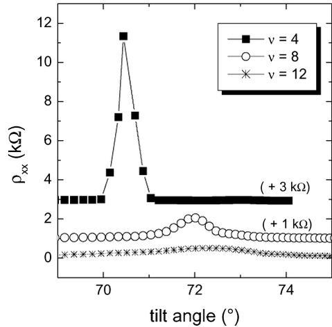
Fig. 2.  $\rho_{xx}$  at filling factors  $\nu = 4N = 4, 8, 12$  as a function of the tilt angle  $\vartheta$ . The maxima occur when two neighboring Landau levels with opposite spin are energetically coinciding. The curves are shifted for clarity.
